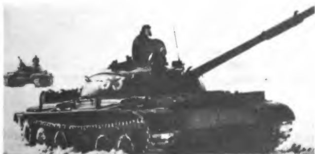
Figure 6-15. T-62 medium tank. The T-62, with a 115-mm smoothbore gun, is replacing the older T-54/55 as the Soviet main battle tank. It can be easily recognized by its five evenly-spaced roadwheels and the bulging fume extractor near the middle of the gun barrel.
